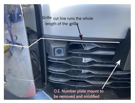
8. When Cutting make sure the grille connecting holes are left intact
