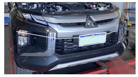
the marked line to allow a perfect fit by back cutting to the desired clearance.
