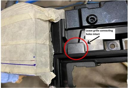
9. Once the bumper cut line is marked you can make the cut using an angle grinder or air saw. Clean edges after cutting and test fit. Set the bumper cut aside now until the bar is fitted.
