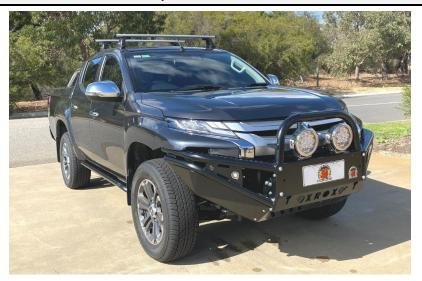
This bar is compatible with the Air Bag system of this vehicle. The compliance label <u>must</u> be attached on a surface of the bar so it can be read and located where it will not sustain environmental damage. The vehicle make and model must be marked on the label with a permanent marker.
