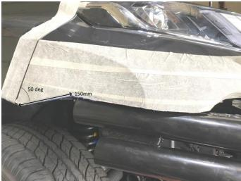
From the start of the bumper at the wheel arch (Point A) Use an angle finder/protractor mark Point B at 150mm along a 50 degree line.
