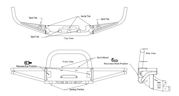
This bar has detachable side wings that can be replaced if damaged; plus 6 spot tab, 3 aerial tabs, 2 jacking positions, 2 recovery eye and 2 hook locations. (Recovery eyes & hooks are not provided in this kit). The bar has been developed to accept up to a 9500Lb. Warn low mount winch.
