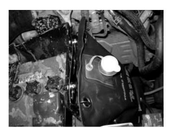
Fasten one end of washer support Bracket to fuel pump bracket. Mark and drill 8mm holes in battery tray to fasten bracket.
