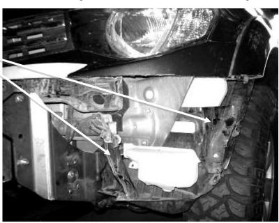
3. **Trim inner guards** and drill 10mm hole as shown in diagram. Utilise an unused inner guard clip to fasten through drilled hole.
