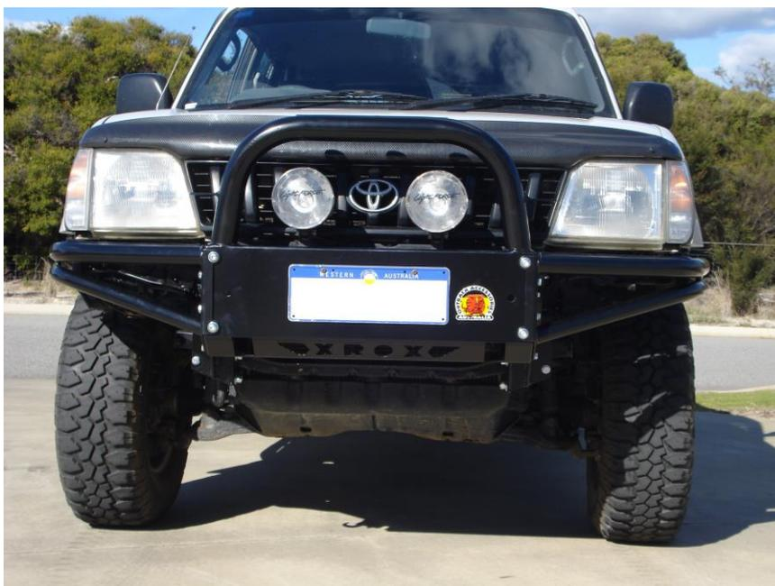
This bar has detachable side wings that can be replaced if damaged; plus 6 spot tab, 3 aerial tabs, 2 jacking positions, 2 recovery eye and 2 hook locations. (Recovery eyes & hooks are not provided in this kit). The bar has been developed to accept up to a 15,000Lb. Warn low mount winch.
