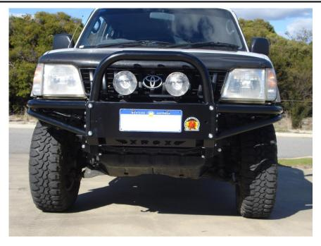
This bar has detachable side wings that can be replaced if damaged; plus 6 spot tab, 3 aerial tabs, 2 jacking positions, 2 recovery eye and 2 hook locations. (Recovery eyes & hooks are not provided in this kit). The bar has been developed to accept up to a 15,000Lb. Warn low mount winch.
