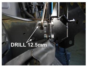
brackets to the mounts using the 10x30 bolts, flat washers, spring washers and nuts. When these are finger tight and clamping the crush can flanges between the mounts and mount supports use a clamp to pull the mount supports hard onto the chassis rail (see figure above) and drill from each side the 4) 12.5mm holes. Fasten the support mounts to the chassis loosely using the 12x120mm bolts, flat washers, spring washers and nuts.
