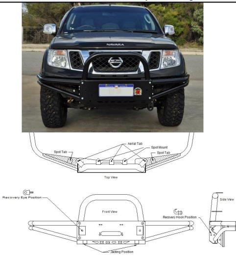
This bar has detachable side wings that can be replaced if damaged; plus 6 spot tab, 3 aerial tabs, 2 jacking positions, 2 recovery eye and 2 hook locations. (Recovery eyes & hooks are not provided in this kit). The bar has been developed to accept up to a 15,000Lb. Warn low mount winch.
