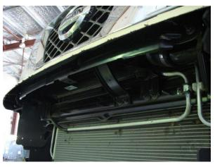
This XROX® tube bar comprises of both **powder coated** and **painted** parts, the side sections and centre are powder coated while the mounts are painted with a zinc enriched satin black enamel. If at any stage through the product's life the painted sections show signs of rusting, remove the rust and recoat with satin black zinc enriched enamel.
