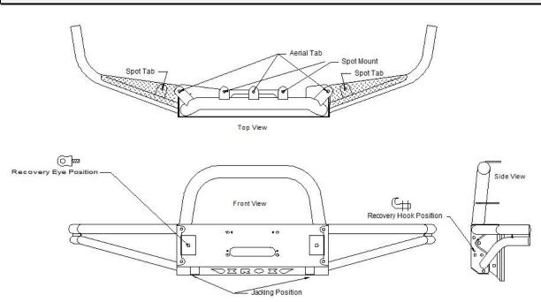
This bar has detachable side wings that can be replaced if damaged; plus 6 spot tab, 3 aerial tabs, 2 jacking positions, 2 recovery eye and 2 hook locations. (Recovery eyes & hooks are not provided in this kit). The bar has been developed to accept up to a 15,000Lb. Warn low mount winch. (*Note: 50mm Lift mounts are available mount ID:XN5*).
