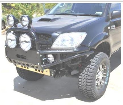
This bar has detachable side wings that can be replaced if damaged; plus 6 spot tab, 3 aerial tabs, 2 jacking positions, 2 recovery eye and 2 hook locations. (Recovery eyes & hooks are not provided in this kit). The bar has been developed to accept up to a 9,600Lb. Warn low mount winch.
