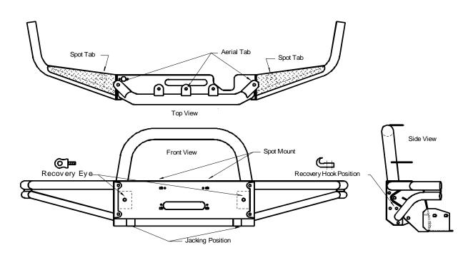
This bar has detachable side wings that can be replaced if damaged; plus 6 spot tab, 3 aerial tabs, 2 jacking positions, 2 recovery eye and 2 hook locations. (Recovery eyes & hooks are not provided in this kit). The bar has been developed to accept up to a 15,000Lb. Warn low mount winch.
