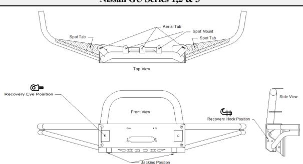
This bar has detachable side wings that can be replaced if damaged; plus 6 spot tab, 3 aerial tabs, 2 jacking positions, 2 recovery eye and 2 hook locations. (Recovery eyes & hooks are not provided in this kit). The bar has been developed to accept up to a 15,000Lb. Warn low mount winch, if fitting a 15,000/12,000Lb winch, the inner bottom part of the grill will need to be cut off to fit this size winch.
