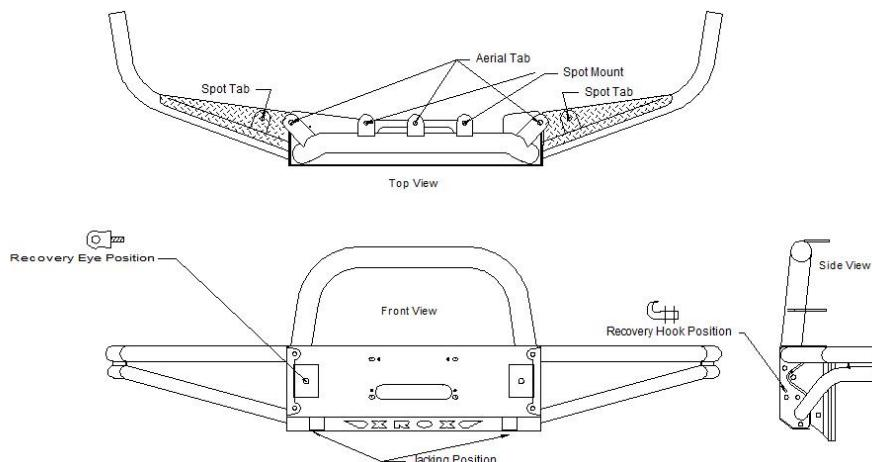
This bar has detachable side wings that can be replaced if damaged; plus 6 spot tab, 3 aerial tabs, 2 jacking positions, 2 recovery eye and 4 hook locations. (Recovery eyes & hooks are not provided in this kit). The bar has been developed to accept up to a 15,000Lb. Warn low mount winch, if fitting a 15,000/12,000Lb winch, the inner bottom part of the grill will need to be cut off to fit this size winch.
