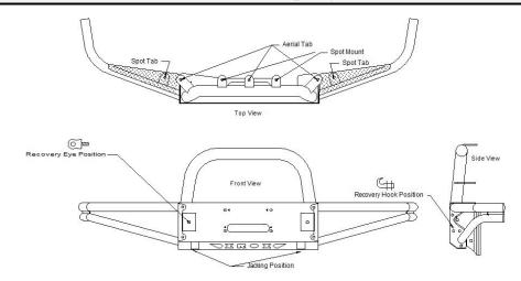
This bar has detachable side wings that can be replaced if damaged; plus 6 spot tab, 3 aerial tabs, 2 jacking positions, 2 recovery eye and 4 hook locations. (Recovery eyes & hooks are not provided in this kit). The bar has been developed to accept up to a 15,000Lb. Warn low mount winch, if fitting a 15,000/12,000Lb winch, the inner bottom part of the grill will need to be cut off to fit this size winch.
