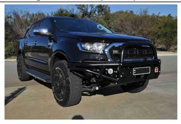
This bar has detachable side wings that can be replaced if damaged; plus 6 spot tabs, 3 aerial tabs, 2 jacking positions and 2 hook locations. (Recovery hooks are not provided in this kit). The bar has been developed to accept up to a 9,500Lb. Warn low mount winch.
