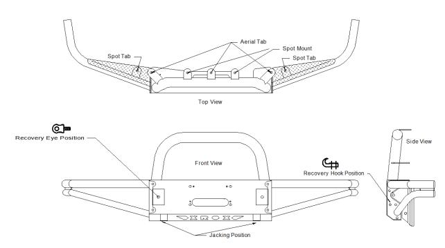
This bar has detachable side wings that can be replaced if damaged; plus 6 spot tab, 3 aerial tabs, 2 jacking positions, 2 recovery eye and 4 hook locations. (Recovery eyes & hooks are not provided in this kit). The bar has been developed to accept up to a 15,000Lb. Warn low mount winch.
