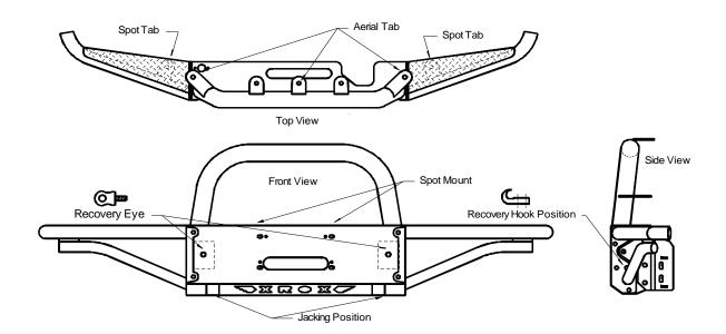
This bar has detachable side wings that can be replaced if damaged; plus 6 spot tab, 3 aerial tabs, 2 jacking positions, 2 recovery eye and 2 hook locations. (Recovery eyes & hooks are not provided in this kit). The bar has been developed to accept up to a 15,000Lb. Warn low mount winch.
