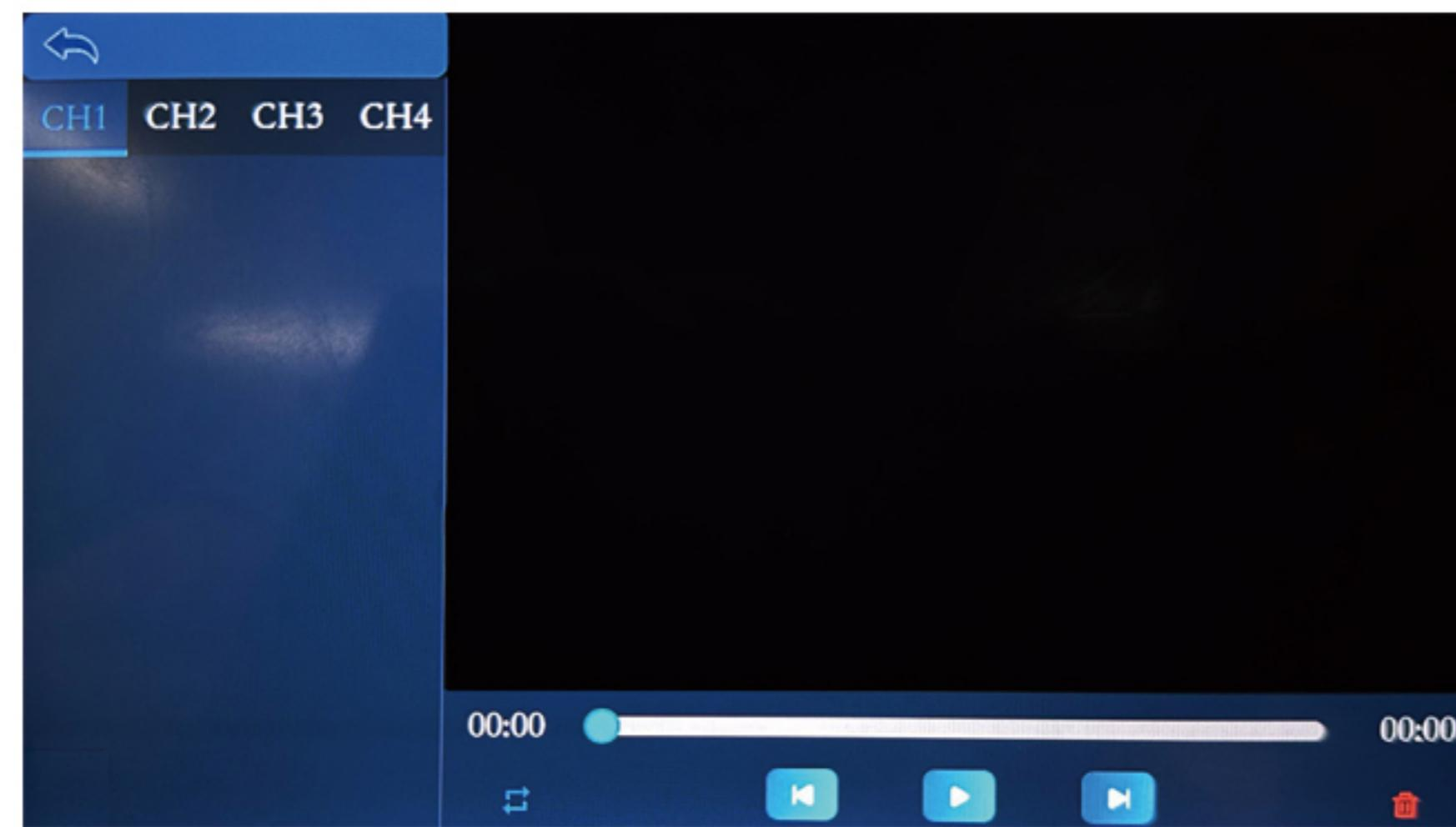
After entering the setting, you can select the channel screen to be viewed by moving **▼▲**, and press CH to confirm.
