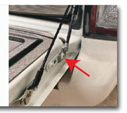
Remove the factory bolt from the hinge closest to the tub and install the strut bracket as shown. Ensure that the lip of the bracket sits under the hinge
