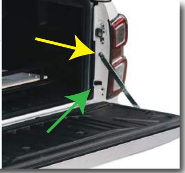
Install the slow down strut. Place the cable on first, followed by the washer. Ensure when tightening, the cable is sitting on the shoulder of the bolt and the cable remains free
