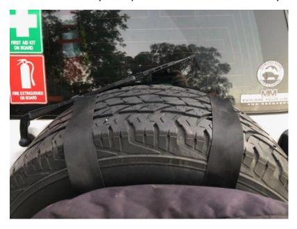
**3.** Feed the straps through from the rear of the wheel/rim to the front.
