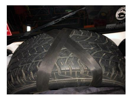
**3.** Pull the straps down behind the tyre and then click the male buckle on the end of each strap into the female buckles, located on the bottom of the Rear Wheel Bag.
