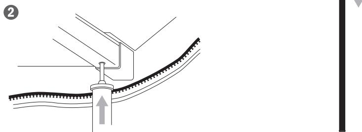
**TIP** IN CASE OF RAIN, LOWER THE SUPPORT LEGS TO ALLOW DOWNWARD SLOPE AND GUY OFF BETWEEN RAFTERS TO FORM VALLEYS FOR WATER RUN-OFF.
