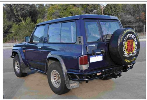
The Xrox<sup>®</sup> Rear Step Tube Bar is designed to give maximum protection to the rear and sides of your vehicle as well as providing a convenient step. It incorporates two Hi-Lift jack positions and has detachable sides that can be replaced if damaged.
