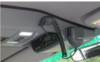
Microphone clip on slight angle
