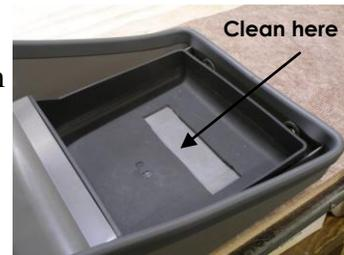
Peel one side of protective backing from foam strip supplied; apply pressure with palm of hand to adhere foam to exposed part of console. Peel backing off other side of foam strip and add one or more strips of foam to suit different size radios (see chart below). This will keep radio level with bottom of surround.
