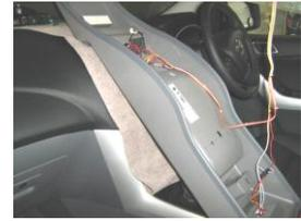
Plug console wiring into interior light wiring of vehicle. Plug **white** wire on console into **white/red** wire of interior light plug. Plug **red** wire on console into **yellow** wire of interior light plug and **yellow** wire on console into **black** wire of interior light plug.
