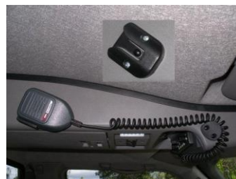
Install microphone clip on acute angle
