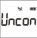
When the LCD is in the off state, press the button to show the current time and connection graph if the product is connected to the smartphone. If disconnected, it will show the disconnection graph. For a paired but disconnected device, it will display "-----." When the product is unpaired, it will show "Uncon." Pressing the button again will switch to mode 1.
