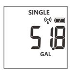
The LCD screen displays "SINGLE" water consumption in liters or gallons. Suppose the flow meter stops running for more than 30 seconds and restarts. In that case, it clears the original accumulated data, begins re-accumulating, and updates the display of real-time water consumption every second.
