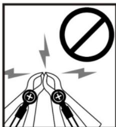
If the leads are connected incorrectly (e.g. Positive on Negative) the Reverse Polarity Protection will cut-in automatically and the REVERSE POLARITY LED will illuminate and the battery charger will switch off.
