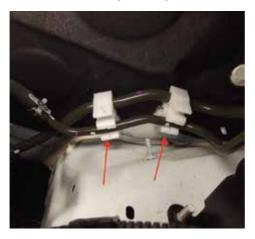
5. Cable tie fuel line to heater hose.
