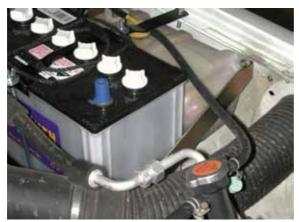
8. Reconnect the negative battery terminal to the main starter battery or install the desired Dual Battery System. Before closing the bonnet make sure the battery, tray and J bolts do not hit the bonnet.
