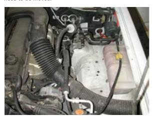
3. Replace the M6 bolts that were removed, bolting the arms of the tray and the washer bottle to the inner guard.
