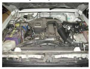
2. Remove the 2xM6 bolts that secure the washer bottle to the inner guard. Place the tray in position against the guard, with the washer bottle remaining in the same place.
