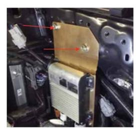
9. Manipulate wiring loom into wedged shaped space between firewall, inner guard and wheel arch to gain clearance for tray.
