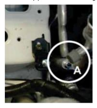
4. Remove A/C bracket from rubber mount on A/C pipe DISCARD.
