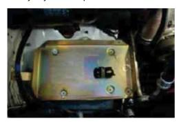
7. Bolt A/C bracket to tray. Use 1xM6 counter-sunk with nut.
