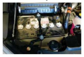
11. Reconnect the negative battery terminal to the main starter battery or install the desired Dual Battery System. Before closing the bonnet make sure the battery, tray and J bolts do not hit the bonnet.
