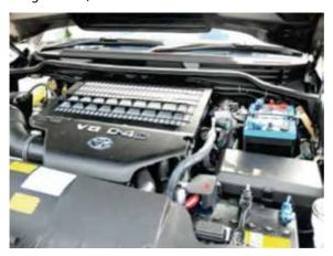
15. Reconnect the negative battery terminal to the main starter battery or install the desired Dual Battery System. Before closing the bonnet make sure the battery and tray do not hit the bonnet.
