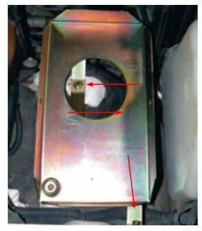
4. Drill 6mm hole for the M6 bolts in the corner of the tray. Fit M6 bolt through the tray with the body washer and nut on the underside of the guard and tighten.
