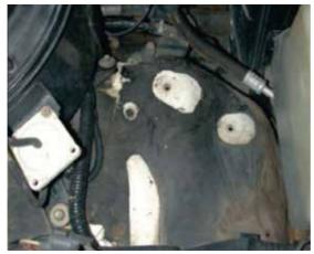
3. Fit the tray in position and hand tighten the 3 x M8 long bolts that secure the tray to the car. Use existing captive nuts on the vehicle.
