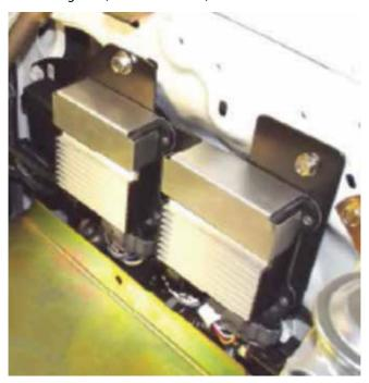
13. Place battery into tray. Secure battery hold down clamp (supplied) with J bolts and fit Long top support mount (supplied). Failure to fit the top mount support brackets may result in your vehicles metal fatiguing and this will void your warranty.
