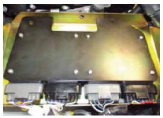
12. Bolt ABS computer mount to inner guard using 1 x M6 bolt (front) and 1 x M8 long bolt (closest to firewall).
