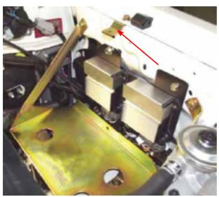
11. Bolt vehicle computers to ABS computer mount (supplied) using original bolt hardware and reconnect wiring plugs as they were removed in point 1.
