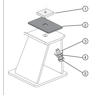
Slide the Rhino Vortex Aero Bar onto M6 Plate Nut as shown and tighten with the 10mm Spanner.
