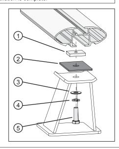
Fix the M6 x 20mm Hex Bolt, both Washers, 2mm HDPE Spacer and M6 Plate Nut onto the EGR post as shown.
