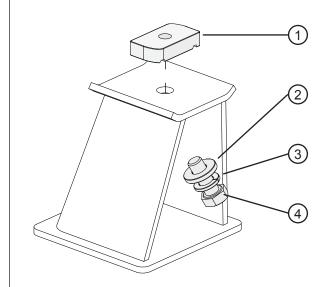
Slide Rhino Heavy Duty Bar onto channel nut as shown and tighten with the 13mm Spanner.
