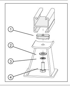
Fix the M8 x 20mm Hex Bolt, both Washers and M8 Channel Nut onto the EGR post as shown. Make sure the channels on the M8 Channel Nut are facing downwards.
