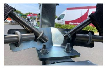
Secure the tubular frames to the rear of the mounting bracket using the small "U-bolts" and fasten.
