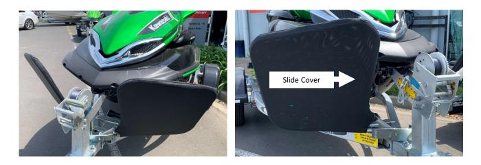
Slide the covers over the tubular frame from the side and secure with zippers running along the inside edge.
