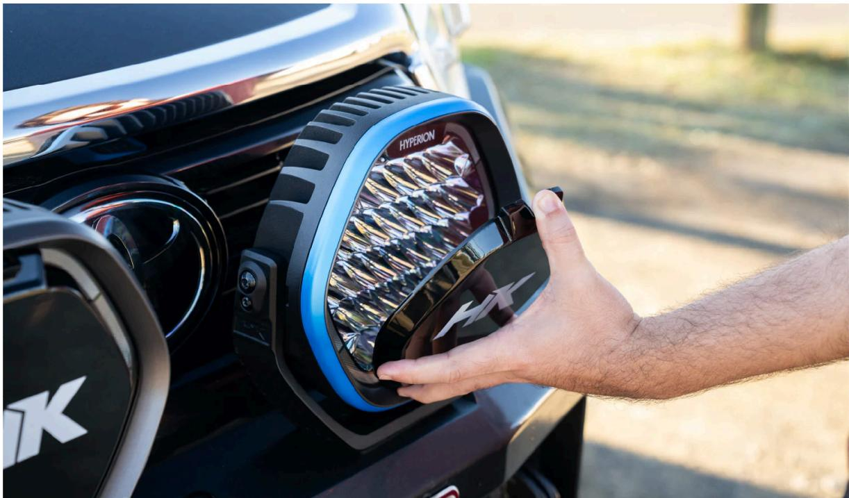
To attach the cover, align the tabs on the bottom of the cover with the corresponding slots at the bottom of the light. Push the top of the cover into the light until you hear a click. This is the top tabs snapping into place.
