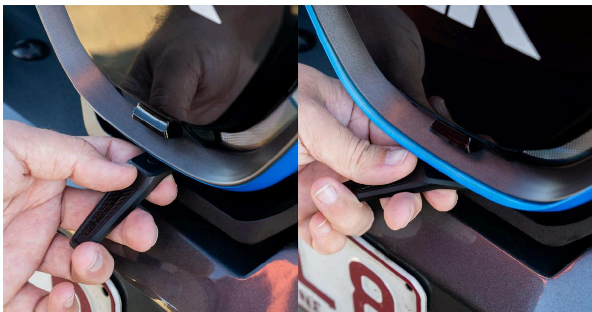
Attaching the accent ring is just as easy, however you'll first want to make sure the ring is in the right orientation. On the back of the accent ring is a T-shaped tab. Position the T-shaped tab at the bottom of the ring, and align it with the slot on the bottom of the light housing. Push the rest of the ring onto the light from bottom to top to attach the ring.
