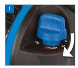
**Step 1.** Slightly depress the control and turn to the LOW position.
