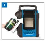
Step 3. Rotate regulator out from heater. Screw the gas cartridge (clockwise direction) onto the gas regulator and tighten securely. Check for leaks with soapy water.
