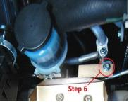
9. Place battery in vehicle fit special top mount with M6 nyloc nut on the "J" bolt closest to the air cleaner. Then drill radiator support panel and bolt top mount using M6 bolt, washer
