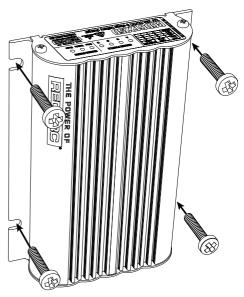
Figure 2.1.1 - Mounting the Charger
