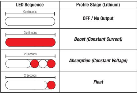
Figure 1.3.2.1 - Charge Stage LED Sequences
