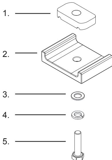
**1** Install the ARB -ASHD Fit Kit hardware in into the ARB Ascent Canopy posts as shown.
