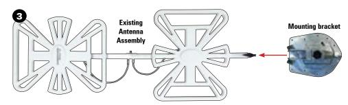
Remove the existing antenna assembly from the mounting bracket.
