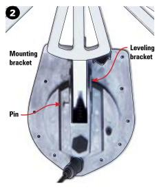
Pull the e-clip off of the pin, and remove the pin from the leveling bracket.
