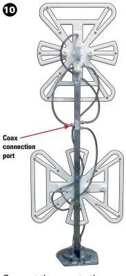
Connect the coax to the coax connection port, and tighten until fingertight. Then, tighten ¼ turn more.
