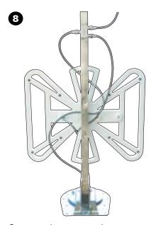
Connect the coax to the coax connection port, and tighten until fingertight. Then, tighten ¼ turn more.
