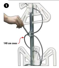
Using a wrench, loosen and remove the 140 cm coax from the coax connection port shown here.
