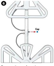
Remove the cap from the coax connection port.
