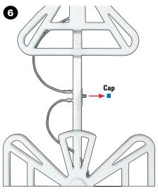
Remove the cap from the coax connection port. Now, install a connector on the end of the coax cable. Refer to the next page for help.
