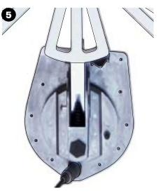
Insert the pin through the leveling bracket and the elevating gear. Push the e-clip over the end of the pin.
