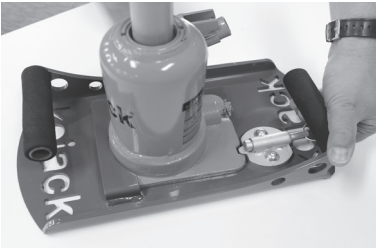
STEP 3 Pull back the pin by holding onto the ring pull as shown
