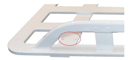
In the desired position, align each mounting point with cross bars on your roof rack. Place the rubber inserts on the inside of each Basket Mounting Brackets, trim where necessary.
