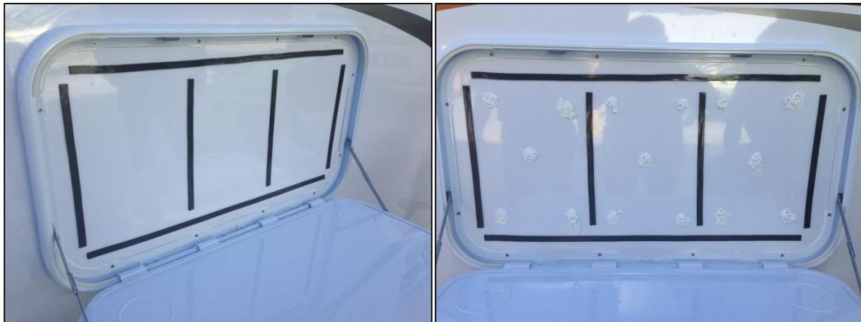
**Step 10:** You are now ready to install the backing plate. Simply align the edges of the backing plate with the internal frame and gently push into position. Please take care in this step as once the double sided tape has adhered, it will be difficult to remove the backing plate to have a second attempt.
