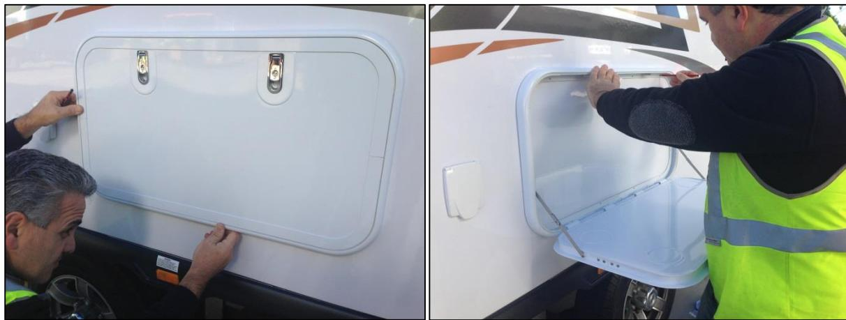
**Step 5:** Once the holes have been marked with a pencil on the side of your vehicle, you are ready to start drilling small pilot holes.
