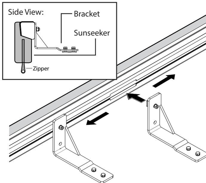
**3** Slide the brackets into the C channel of the crossbar using the installed Plate Nuts. Tighten with a 13mm socket wrench. Check all fixtures are secure before driving.
