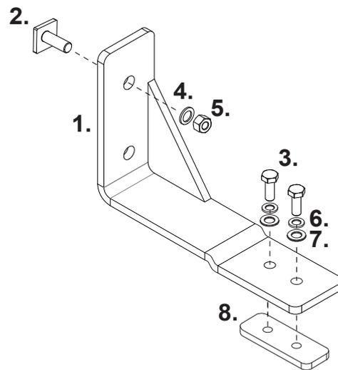
**2** Insert the bracket assemblies into the Sunseeker as shown.
