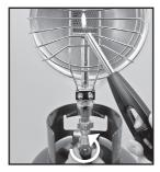
2. If the burner head has not ignited, turn the cylinder gas control valve to the off position, wait for 1 minute then repeat the previous step.
