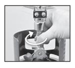
2. Loosen the connection to the gas cylinder in a clockwise direction.
