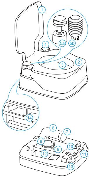
1 Cover • 2 Seat • 3 Toilet bowl • 4 Water filler cap • 5a Piston pump • 5b Bellow pump • 6 Pour out spout • 7 Cap pour out spout • 8 Lip seal • 9 Vent seal • 10 Vent button • 11 Valve handle • 12 Storage for toilet fluids • 13 Level indicator waste-holding tank (dependent on model) • 14 Clasp
